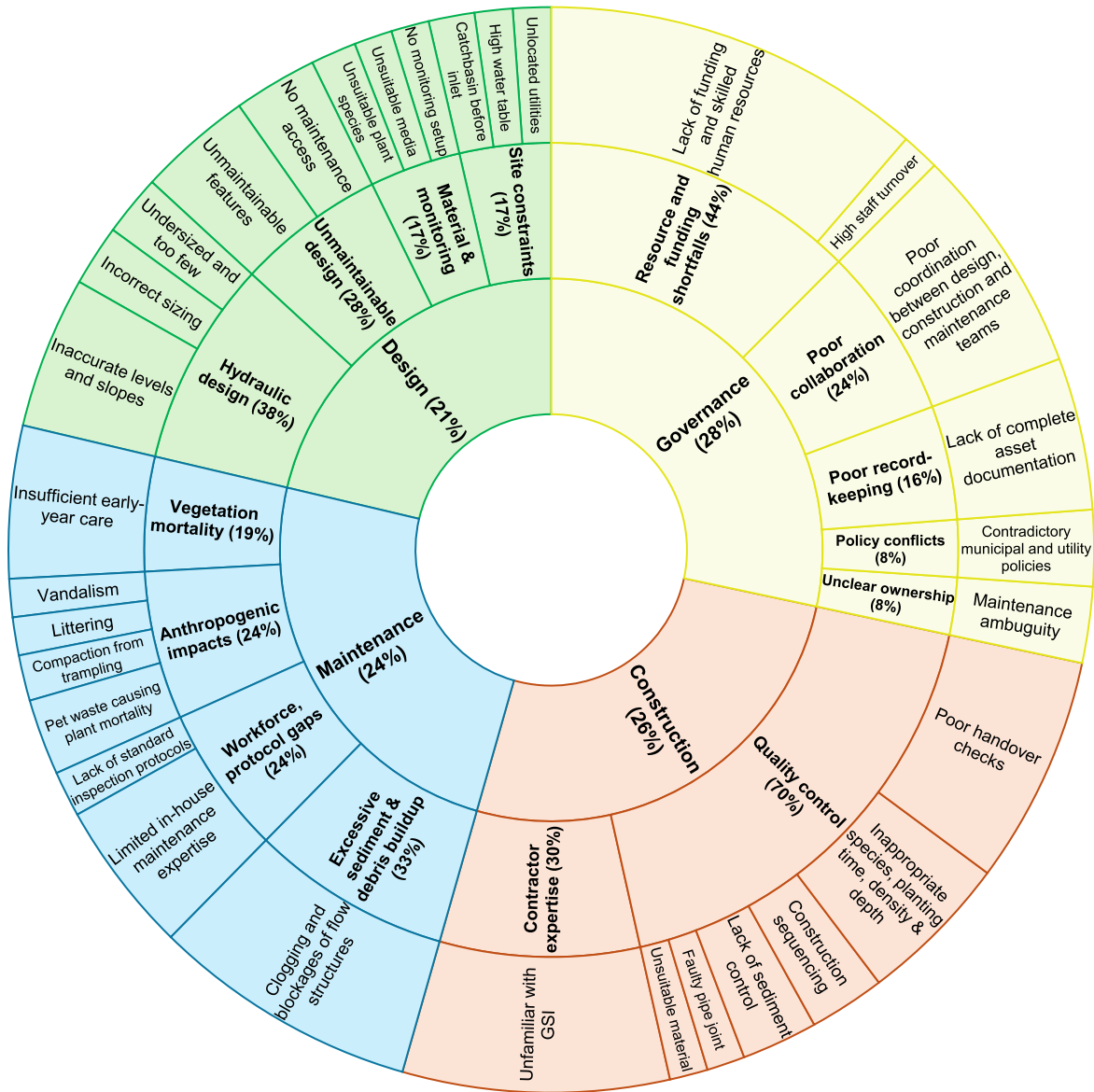
Figure 1. Recurring design, construction and maintenance issues in the roadside GSI asset
